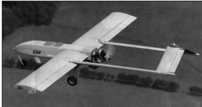
The Tactical Unmanned Aerial Vehicle (TUAV) system is designed as a ground maneuver commander's primary day/night reconnaissance, surveillance, target acquisition, and battle damage assessment system.
