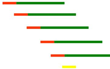
The maintenance schedules of five of the units are shown by the red bars in the figure and allow for extra maintenance if necessary. The sixth unit operates in the times indicated by the red bars, and the sixth unit is maintained at the time indicated by the yellow bar.
