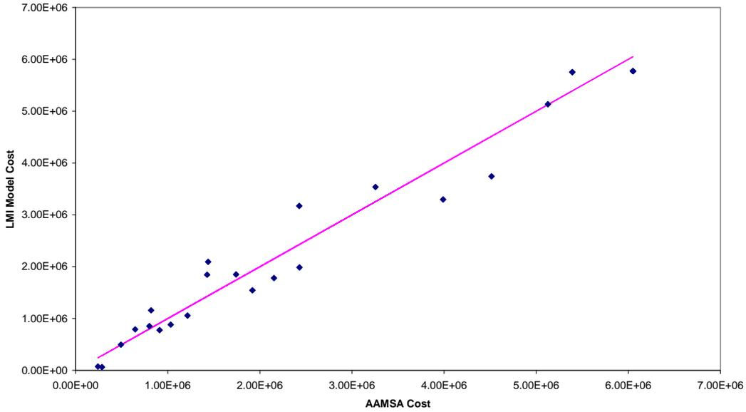
The mean absolute deviation of the model from the data is 19 percent. That is, the model predicts the AMSAA cost information with an average error of 19 percent. We find that fact, and the general appearance of the results shown in the figure, encouraging. The reliability improvement/cost model for the TAAF period is able to reproduce AMSAA data reasonably well.
