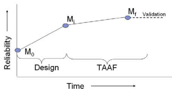
We address the design and TAAF periods below. We begin with the TAAF period because the design-period model uses concepts from the TAAF-period model.
