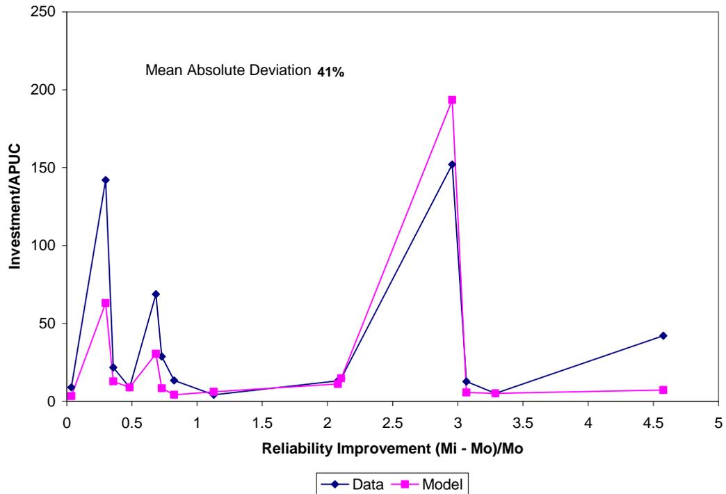
We are cautiously encouraged by the result. The model captures the trend of cost as a function of improvement reasonably well, and it treats data from two distinct platforms consistently. (The AIM-9X datum, the second point from the right in Figure C-2, is not an outlier, but happens to be one of the best-fit points.)
