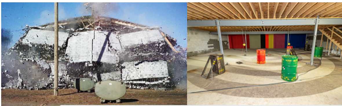
Figure 14. Two-story over-burial building debris test conducted in partnership with the U.S. Army Aberdeen Test Center, Maryland
