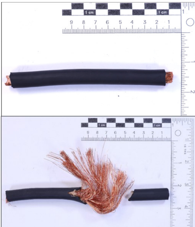
Figure 3. Wire Bundle Target Examples Before and After Test
