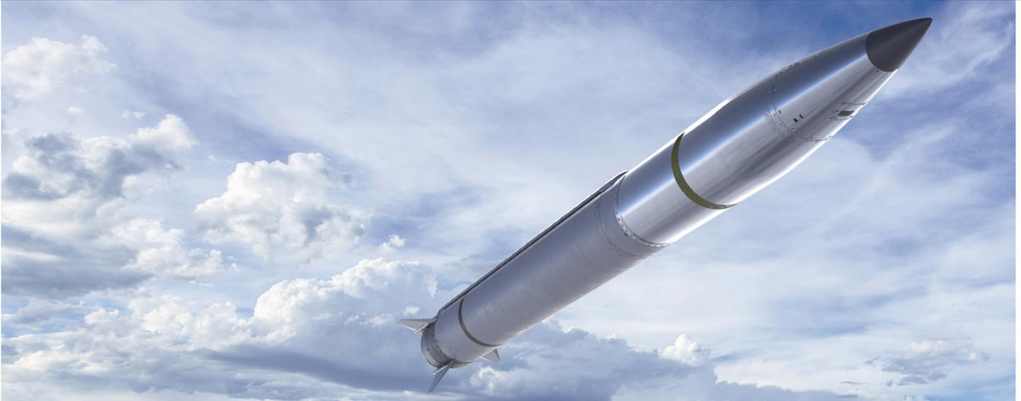
In October 2023, the Army executed three system qualification test (SQT) shots of the Extended Range Guided Multiple Launch Rocket System (ER GMLRS). The program continued to experience reliability failures with the new side-mounted proximity sensor (SMPS), predominantly on the ER GMLRS Alternative Warhead (AW) variant. The SMPS enables an optimal height of burst (HOB) for both the ER GMLRS AW and Unitary warhead variants.
