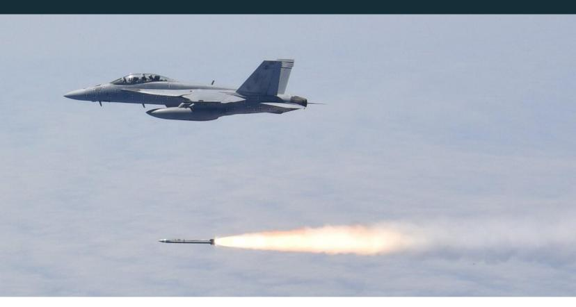
The Navy has completed six developmental test (DT) shots (DT1-DT6) since FY21 for the AGM-88G Advanced Anti-Radiation Guided Missile – Extended Range (AARGM-ER), to identify and fix problems before beginning integrated operational testing. The Navy executed three developmental free-flight tests in FY23 from F/A-18Fs in November 2022 (DT4), April 2023 (DT5), and July 2023 (DT6). AARGM-ER IOT&E free-flight tests are scheduled to begin in 1QFY24.
