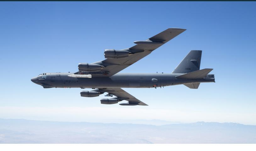
Modification of B-52 Radar Modernization Program (RMP) test aircraft and development of initial system flight software began in FY23. Developmental and integrated flight testing is planned to begin in FY25 leading to IOT&E, full-rate production, and operational fielding in FY27.
