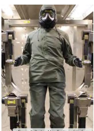
Figure 1. Porton Man Testing of Uniform Integrated Protective Equipment
