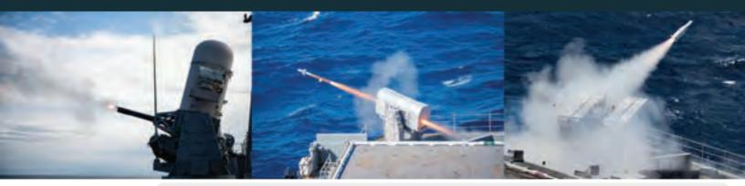
Air Warfare Ship Self-Defense components include, from left to right: Close-in Weapons System, Rolling Airframe Missile, and Evolved Sea Sparrow Missile
