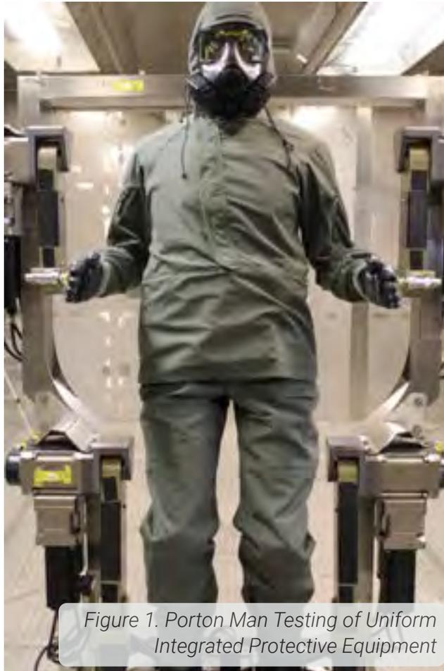
*Figure 1. Porton Man Testing of Uniform Integrated Protective Equipment*
