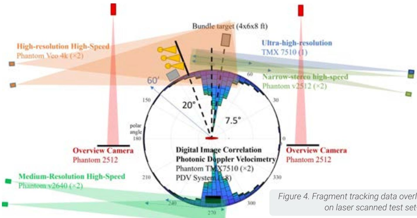
Figure 4. Fragment tracking data overlaid on laser scanned test set-up
