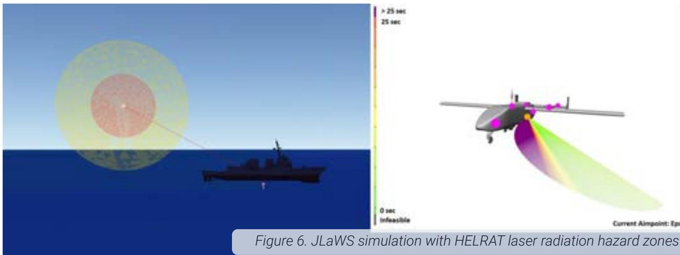
Figure 6. JLaWS simulation with HELRAT laser radiation hazard zones
