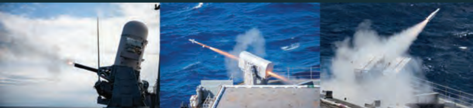
Air Warfare Ship Self-Defense components include, from left to right: Close-in Weapons System, Rolling Airframe Missile, and Evolved Sea Sparrow Missile
