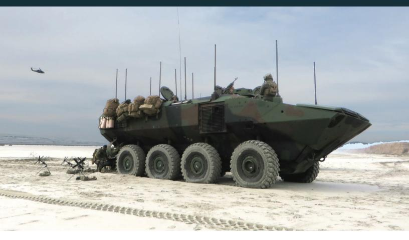
The U.S. Marine Corps regiment or battalion command group equipped with the Amphibious Combat Vehicle – Command and Control variant (ACV-C) is operationally effective as a stationary command post. The ACV-C is suitable and survivable to most threshold ballistic threats. It is vulnerable to cyberattack from nearsiders with physical access to the ACV-C.
