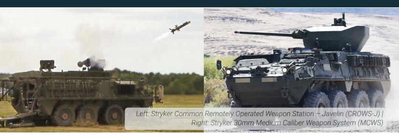
The Army has not verified through testing that the issues identified in the November 2021 FOT&E report on the Stryker Common Remotely Operated Weapon Station – Javelin (CROWS-J) have been resolved. The Army should convene a failure review board, continue CROWS-J corrective actions, and evaluate unit performance in a subsequent FOT&E.
