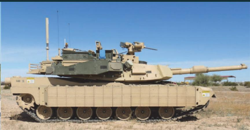
The Army tested the TROPHY Active Protection System (APS) installed on Abrams M1A2 System Enhancement Package version 3 (SEPV3) tanks in FY22 to inform an urgent materiel release (UMR). The TROPHY APS intercepted most of the incoming threats and the Abrams tank base armor provided adequate force protection.
