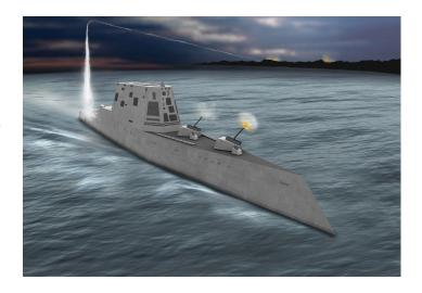
• MK 57 Vertical Launch System (VLS) – The DDG 1000-only vertical missile launcher variant.
