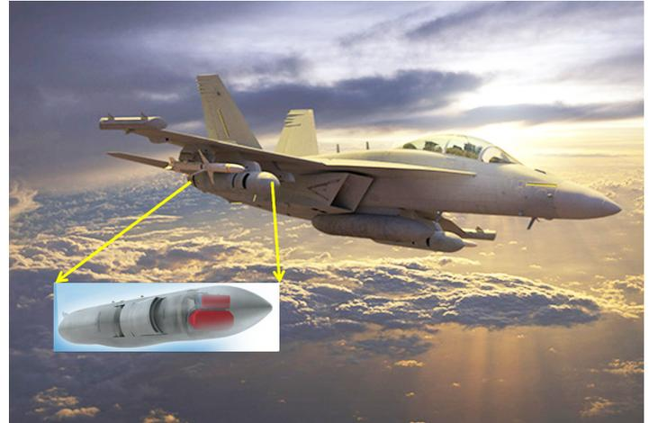
this with greater Effective Isotropic Radiated Power (EIRP) and four active electronically scanned arrays.
