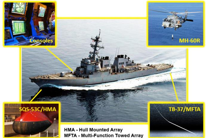
HMA - Hull Mounted Array
