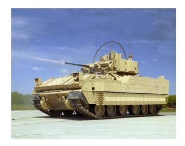
• The A4 versions will inherit the survivability enhancement features found on the A3/ODS-SA baseline configurations: Bradley Urban Survivability Kits, Bradley Reactive Armor Tiles, and Add-on Armor Kit that the Army developed and fielded in response to Operational Needs Statements during Operation Iraqi Freedom. The A4 will include the Commander's Independent Viewer.
