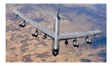
• The B-52H CERP replaces the legacy TF33 engines with fuel-efficient, commercial-derivative engines, increases electrical power generation capacity, and integrates digital engine controls and displays.
