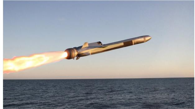
to integrate the OTH-WS on the guided-missile frigate, FFG(X). The OTH-WS will receive targeting data via tactical communications from combatant platforms or airborne sensors and requires no guidance after launch.
