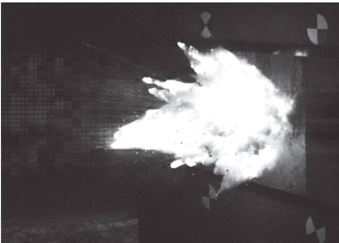
Figure 10. High-speed Image of BAD Fragments Resulting from an EFP
