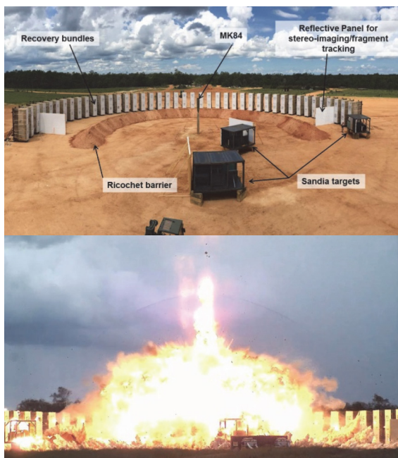
Figure 4. MK 84 Vertical Arena Test: Arena Setup (top); Still Image from High Speed Video after Detonation (bottom)
