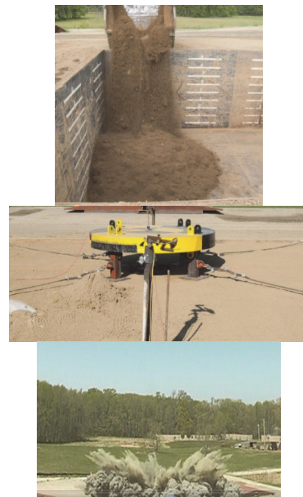
Figure 7. UBB Live Fire Test: Soil Being Placed in Test Box (top); Test Bed Complete (middle); Detonation (bottom)
