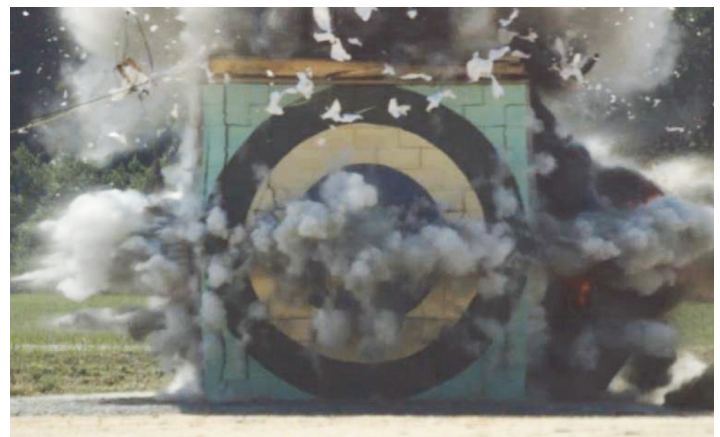
Figure 5. Still Image from Concrete Masonry Unit Building Debris Characterization Test
