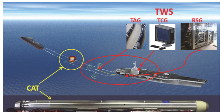
CAT - Countermeasure Anti-Torpedo RSG - Ready Stow Group TAG - Target Acquisition Group TCG - Tactical Control Group TWS - Torpedo Warning System
