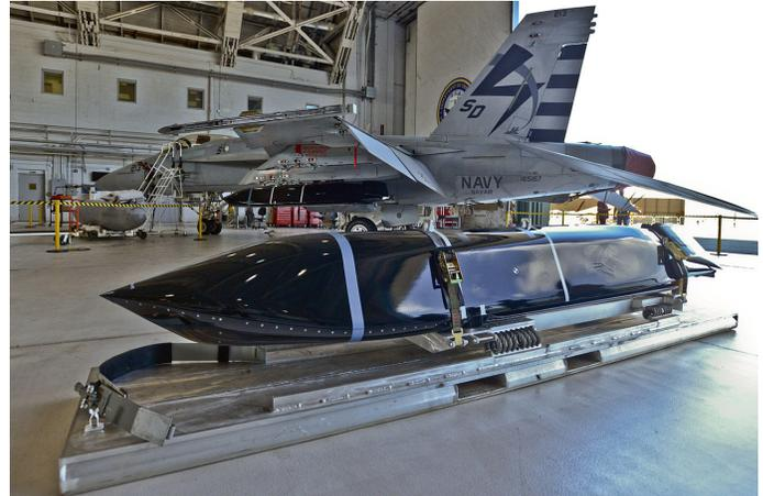
provided to the missile by the launch platform until the RFS identifies and locates the target ship. The missile will then home on the target ship until the IR seeker is able to detect and track the target. The IR seeker will provide terminal guidance to the selected aimpoint on the ship. LRASM is designed to operate individually or as part of a salvo.
