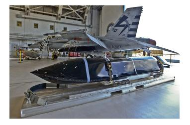
provided to the missile by the launch platform until the RFS identifies and locates the target ship. The missile will then home on the target ship until the IR seeker is able to detect and track the target. The IR seeker will provide terminal guidance to the selected aimpoint on the ship. LRASM is designed to operate individually or as part of a salvo.
