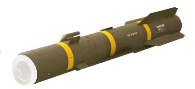
• The HELLFIRE Romeo warhead Integrated Blast and Fragmentation Sleeve (IBFS) detonates with a programmable delay fuse and a Height-of-Burst (HOB) feature. This updated warhead blast provides a capability to engage armored vehicles while the IBFS and HOB feature engage personnel in the open. The programmable delay allows time for the warhead to penetrate deep into a building, bunker, or lightly armored vehicle before detonating to incapacitate the personnel and destroy the equipment inside.
