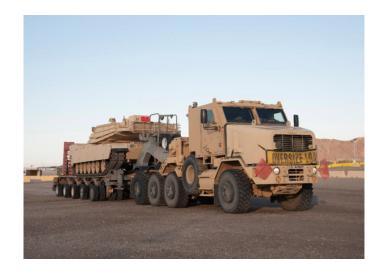
rails of the vehicle chassis. The cab can accommodate six soldiers: the driver, the assistant driver, and four crew of the transported vehicle.
