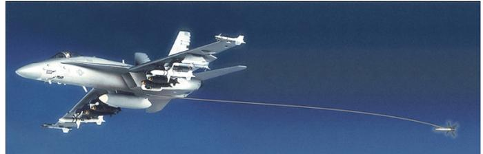
off-board fiber-optic towed decoy that is more integrated with the ALQ-214.
