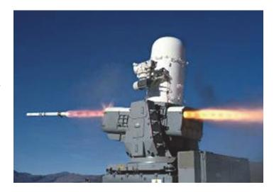
SeaRAM, as used on selected DDG 51-class ships, can launch the RAM Block 2 that incorporates changes to improve its kinematic capability and its capability to guide on certain types of ASCM radio frequency threat emitters in order to defeat newer classes of ASCM threats
