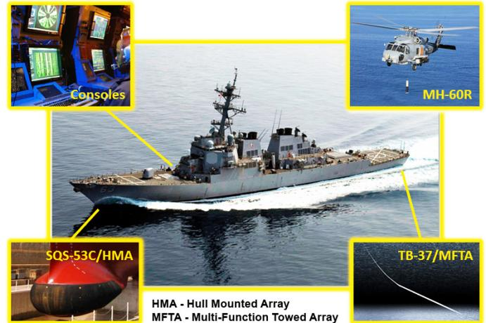
HMA - Hull Mounted Array
