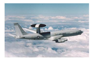
suite includes ultra high frequency, very high frequency, high frequency radios, satellite communications; and Link 16 and Link 11 tactical datalinks. The E-3 AWACS Block 30/35 upgrade included an Electronic Support Measures (ESM) system – passive detection of electronic signals – mounted on the cheeks of the airframe, under the nose, and in the tail.
