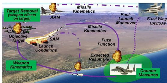
**Figure 2. The primary J-ACE interface is through the Joint Anti-Air Model (JAAM). JAAM is a fast running simulation of Air-to-Air Missiles (AAM) and Surface-to-Air Missiles (SAM); and, aircraft aerodynamic performance.**
