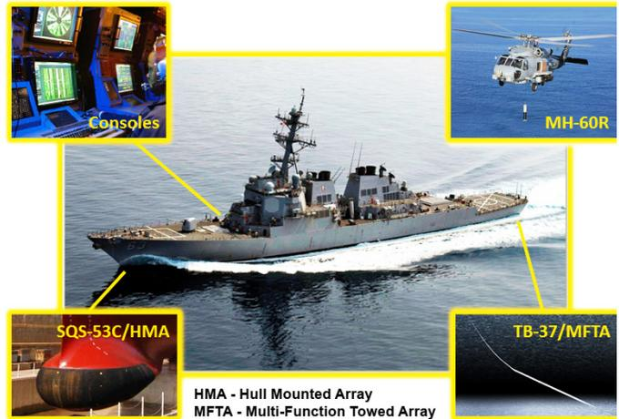
HMA - Hull Mounted Array
