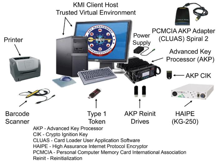
Key Processor for autonomous cryptographic key generation and a Type 1 user token for role-based user authentication. The commercial off-the-shelf components include a client host computer with monitor and peripherals, High Assurance Internet Protocol Encryptor (KG-250), printer, and barcode scanner.
