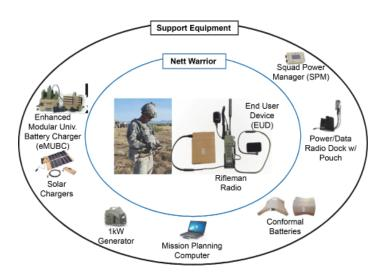
and enemy activity on a digital geo-referenced map image. Nett Warrior is connected through a secure radio to the Soldier Radio Waveform network to communicate among different echelons using voice, data, and position location information messages.
