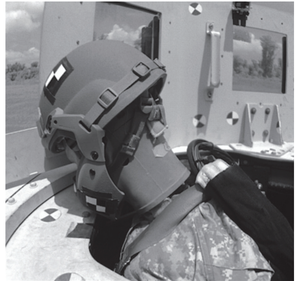
Helmet with Mandible Protection under Test
