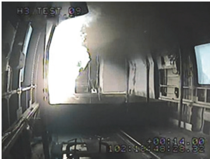
Crew Compartment Fire Testing
