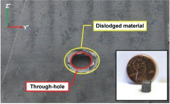
AHEAD sub-projectile and its damage
