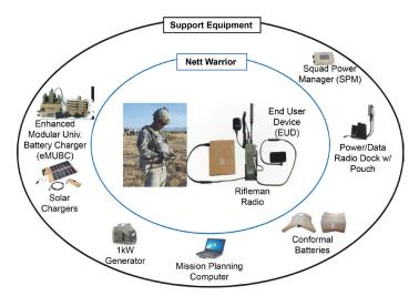
messages, and enemy activity on a digital geo-referenced map image. The Nett Warrior is connected through a secure radio to the Soldier Radio Waveform (SRW) network to communicate among different echelons using voice, data, and position location information messages.
