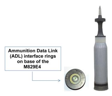
The visible difference between the two cartridges is the Ammunition Data Link (ADL) interface rings on the base of the M829E4. The rings serve as the interface between the Abrams' fire control system and the M829E4. The ADL enables the Abrams' fire control system to send information to the M829E4.
