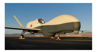
sensor provides full motion video and still imagery of surface targets. An Electronic Support Measures system detects, identifies, and geolocates radar threat signals. An Automatic Identification System receiver permits the detection, identification, geolocation, and tracking of cooperative vessels equipped with Automatic Identification System transponders.
