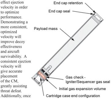
a desired ejection velocity is obtained and parameters that affect it are identified, a common impulse cartridge for all Services will be more easily achievable, thereby reducing support costs. In the next phase, NSWC-Crane will conduct a flight test to determine how tailored flares improve effectiveness. Methods to adjust ejection velocity will be used to enhance effectiveness of current expendables.
