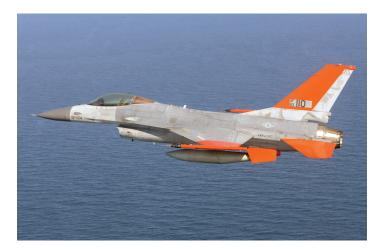
• The QF-16 retains F-16 flight performance characteristics and payload capabilities including supersonic, after-burning engines, high-G maneuvering, complex electronic attack, and expendable countermeasures.
