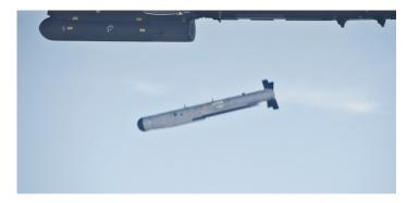
• SDB provides reduced collateral damage while achieving kills across a broad range of target sets by precise accuracy, small warhead design, and focused warhead effects.
