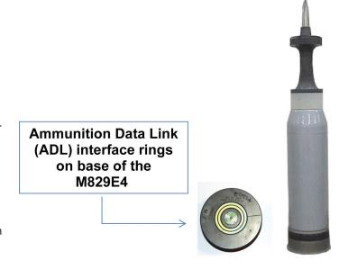
The visible difference between the two cartridges is the Ammunition Data Link (ADL) interface rings on the base of the M829E4. The rings serve as the interface between the Abrams' fire control system and the M829E4. The ADL enables the Abrams' fire control system to send information to the M829E4.
