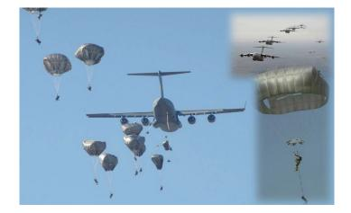
system uses a drogue/sleeve and a mesh slider to control the rate of canopy opening and minimize aircraft exit interference problems. The T-11 replaced the T-10 parachute.
