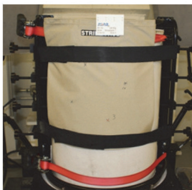
Thoracic test devices representing human torso for evaluating blunt trauma behind body armor. (UK version on left, Canadian on right)
