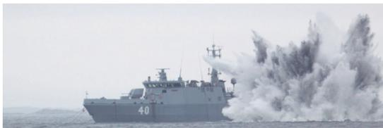
Combat Ships, and the Navy International Program Office. Of particular interest to JLF-Sea were Navy efforts to reduce the cost of shock trials. A new instrumentation scheme that used existing network connections to connect each recording station was proposed and demonstrated. The approach significantly
