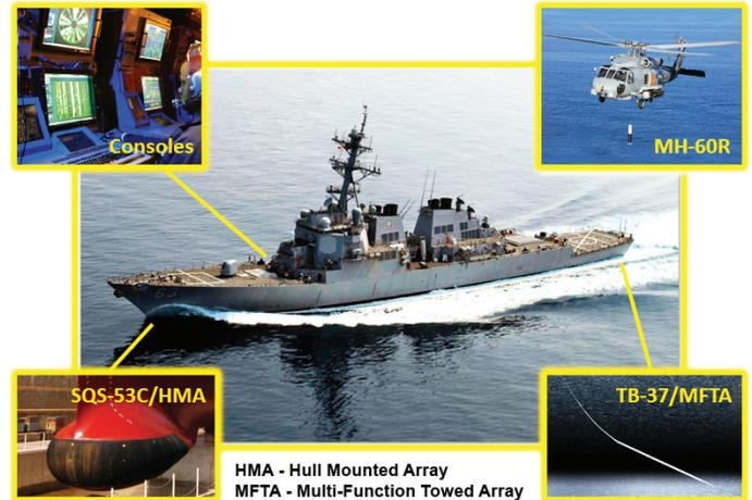
HMA - Hull Mounted Array
