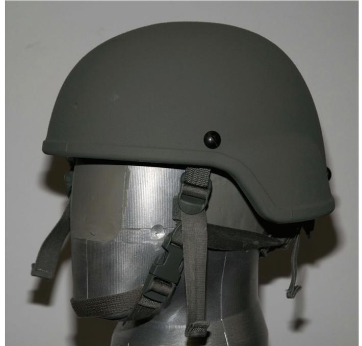
using ultra-high-molecular-weight polyethylene fibers. Unlike aramid composites, the ultra-high-molecular-weight polyethylene ballistic material absorbs ballistic impact and dissipates energy via extensive plastic strains. This results in more resistance to penetration but it also results in large permanent helmet shell deformations and larger damaged areas following impact for a wide range of ballistic threats.
