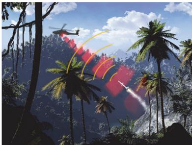
**Multi-Digital Radio Frequency Memory (DRFM) Coherence for Self-Protection and Escort Jamming.** The Naval Research Laboratory is developing algorithms to demonstrate a DRFM jammer pair that operates in concert, but without any link between two independent jammers. Once the algorithms are
