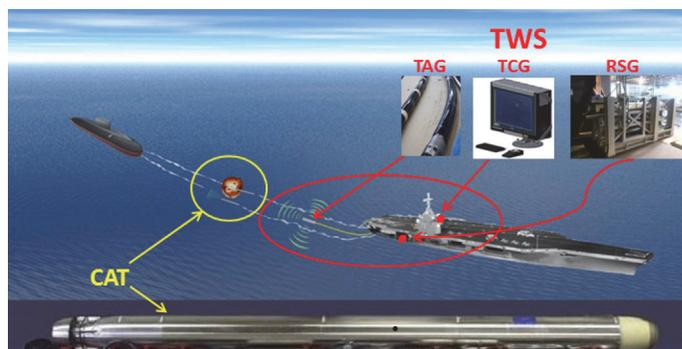
CAT - Countermeasure Anti-Torpedo Torpedo
