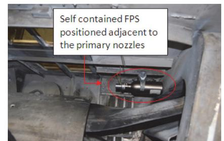
both detection of the fire within 4 microseconds, and suppression within 500 microseconds. In addition, the system will be rechargeable and contained within a single unit.
