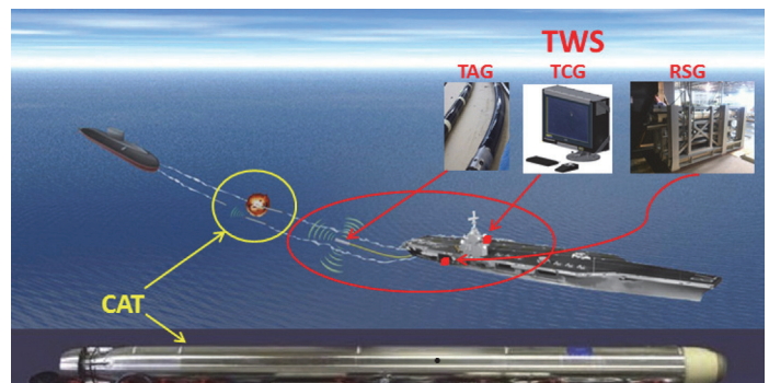
CAT - Countermeasure Anti-Torpedo Torpedo RSG - Ready Stow Group TAG - Target Acquisition Group TCG - Tactical Control Group TWS - Torpedo Warning System
