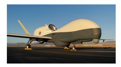
electro-optical/infrared sensor provides full motion video and still imagery of surface targets. An Electronic Support Measures system detects, identifies, and geo-locates radar threat signals. An Automatic Identification System (AIS) receiver permits the detection, identification, geo-location, and tracking of cooperative vessels equipped with AIS transponders.
