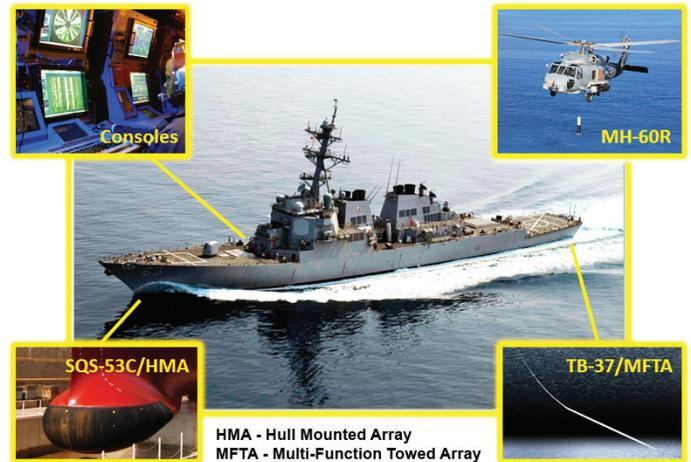
HMA - Hull Mounted Array
