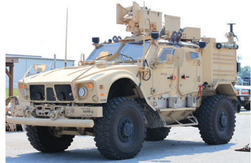
Special Operations Forces MRAP All-Terrain Vehicle (M-ATV) with Underbody Improvement Kit (UIK)
