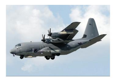
features include the AN/ALR-56M radar warning receiver, AN/AAR-47(V)2 missile warning system, and AN/ALE-47 countermeasures dispensing system. Vulnerability reduction features include fuel system protection (fuel tank foam to protect from ullage explosion), redundant flight critical components, and armor for crew and oxygen supply protection.
