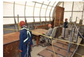
The objective of this project, jointly funded by the Office of Naval Research and JLF, is to validate injury response functions developed under an earlier JLF project. Three Hybrid-III ATDs were tested on a floating shock platform to collect data on personnel injuries caused by an underwater explosion. The data and observations from this testing will improve the accuracy of crew casualty predictions made as a part of ship live fire vulnerability assessments.
