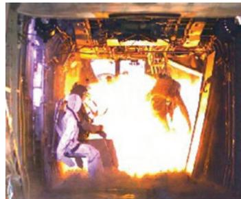
developed under this project, data were collected using a comprehensive instrumentation package gathering multiple temperature, oxygen and carbon monoxide levels, and visibility measurements. For each test event, the cause and time to reach an incapacitation threshold were determined.
