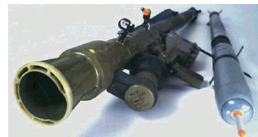
The JASP, in conjunction with the Naval Research Laboratory (NRL), is performing in-depth analyses of newly obtained threat infrared seekers to develop flare and jammer infrared countermeasures (IRCM). The first objective is to identify
