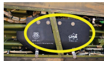
AH-1Z Complex Shape Armor Installation
