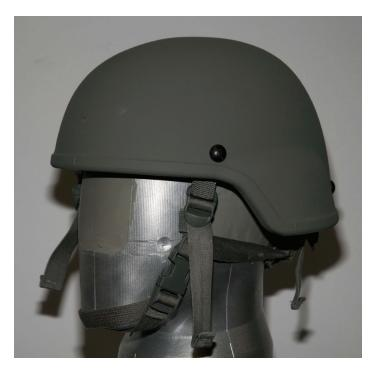
The ECH consists of a ballistic protective shell, a pad suspension system, and a 4-point chin strap/nape strap retention system. Unlike the ACH and LWH helmets, which are constructed with aramid fibers, the ECH is constructed using ultra-high-molecular-weight polyethylene fibers.
