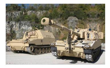
M109A6 howitzer fleet. The full-rate production howitzers will have a newly designed hull, modified Bradley Fighting Vehicle power train and suspension, and a high-voltage electrical system. Operated by a crew of 4, the howitzer is capable of achieving ranges of 22 kilometers using standard projectiles and 30 kilometers using rocket-assisted projectiles.
