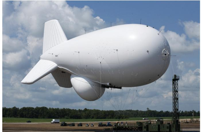
tethered aerostat balloons that operate at altitudes up to 10,000 feet above mean sea level.
