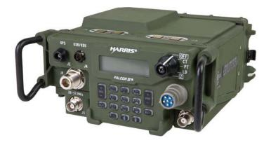
Internet Protocol (VoIP) and digital data on a single channel. Digital data include file transfers, chat, streaming video, and position location reports. ANW2 allows units to use internet protocol routing to transmit medium to high bandwidth data traffic over tactical Very High Frequency, Ultra High Frequency, and L-band radio networks.
