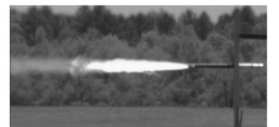
already used for U.S. missile systems testing. Essentially, the missile flies towards the target guided by “ropes” that are cut just feet before impact, allowing natural thrust and fuzing, yet controlling the guidance. Initial testing in FY11 demonstrated an impact accuracy of approximately 3 inches.
