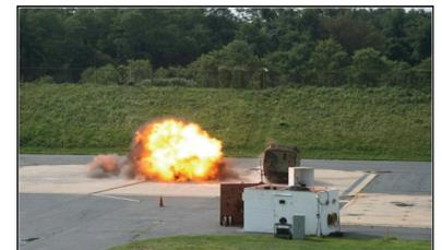
Engineers will use the data to develop lethal-miss-distance contours (the distance from a detonation that a person or equipment must be to survive) with respect to mobility, firepower, and catastrophic target kills.
